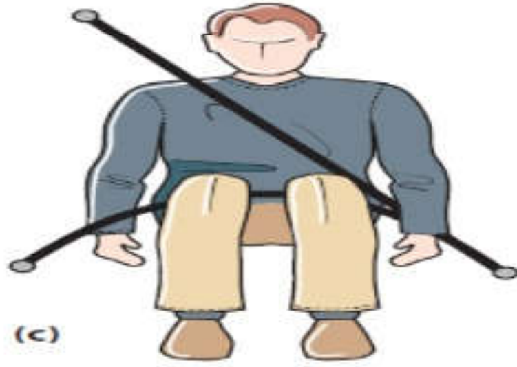
Figure 9.13 Types of seatbelt restraint: (a) simple lap-strap (dangerous to aorta); (b) diagonal only (can slip underneath); (c) diagonal plus lap-strap (usual car type); and (d) shoulder harness (used in aircraft and racing cars).
